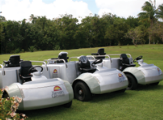
Electric trams specified and designed during the Harrison’s Detailed Design Project for use in the environmental sensitive Harrison’s Cave. Photo: Steve Devonish
